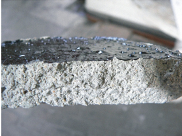
Figure 1: Non-penetrating effect of an 'oil-in-water' bitumen emulsion
