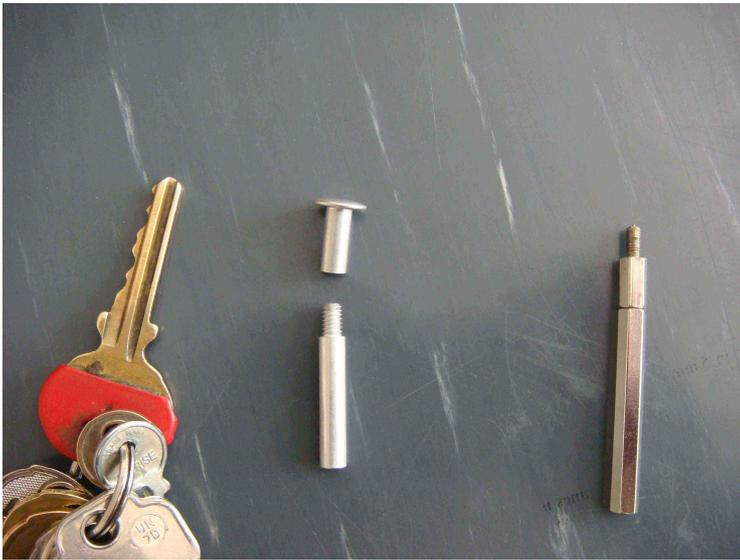
**Figure 6: Pins used for monitoring settlement/deformation below the asphalt layer.**
