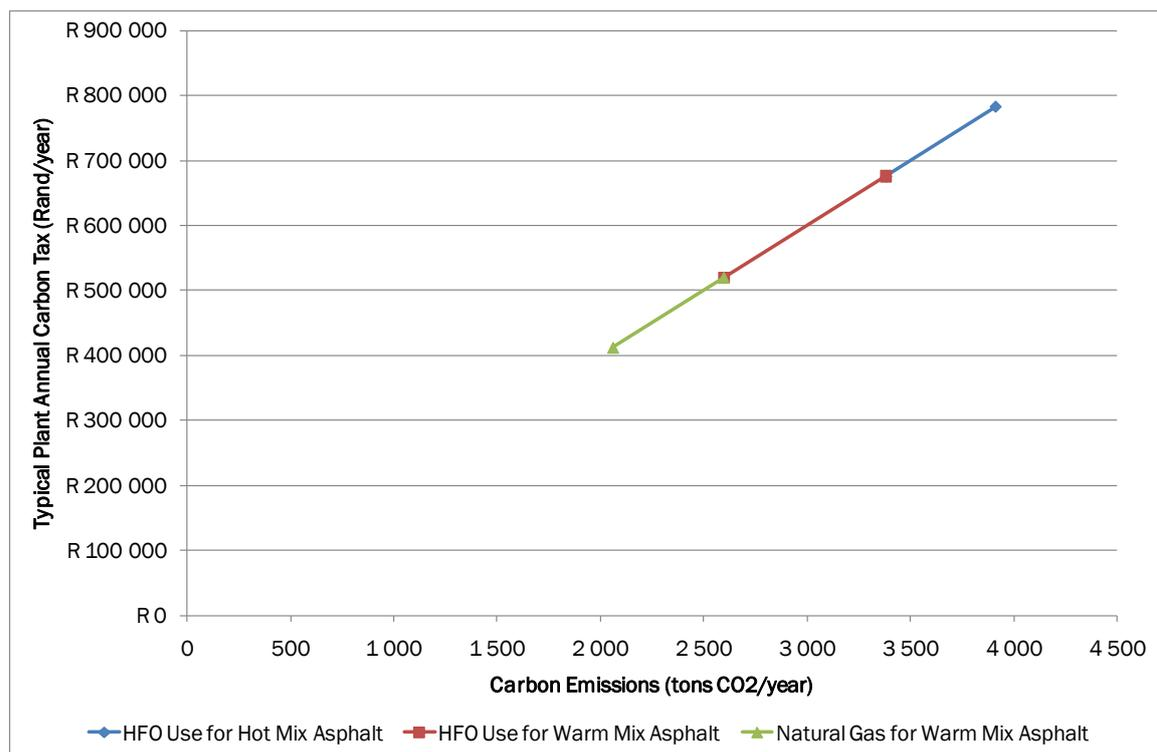
Figure 2: Reducing dryer/mixer CO<sub>2</sub> emission via switch to WMA & burner fuel changes
