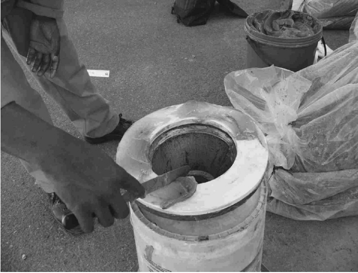
Figure E3: Applying grease to the spacer of the apparatus
