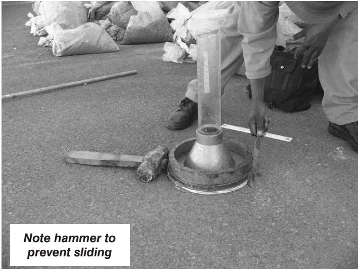
Figure E6: Applying grease to outer edge
