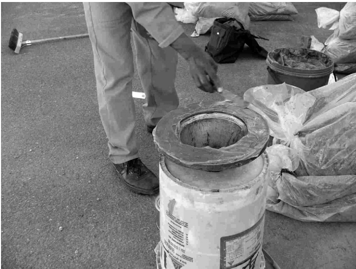
Figure E2: Applying grease to the base of the apparatus
