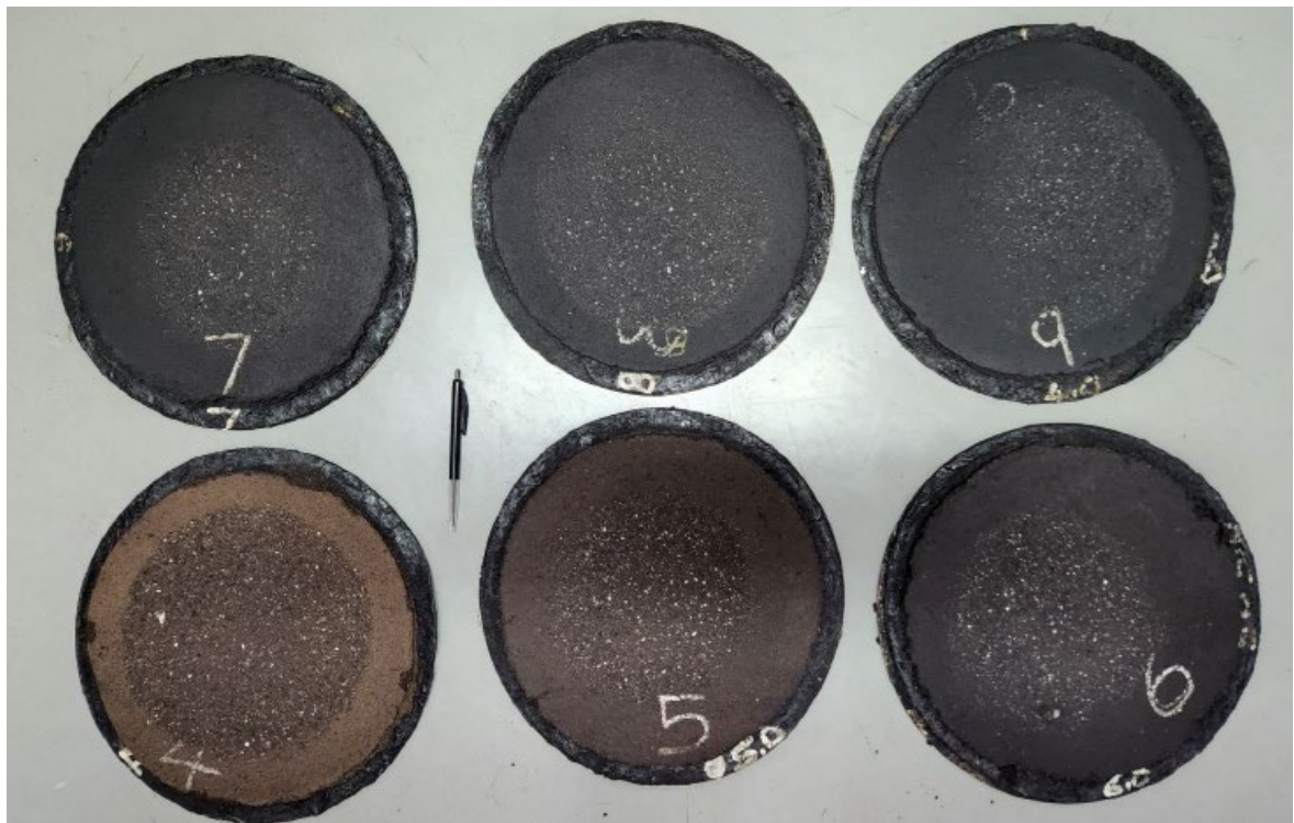
Figure 29 Fine slurry (Medium grading) - Specimens after WTAT
