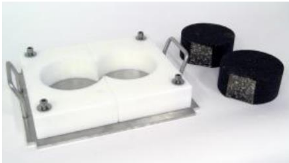
Figure 1: Cut Face Cores/Specimens and Specimen Mounting Mould /System
