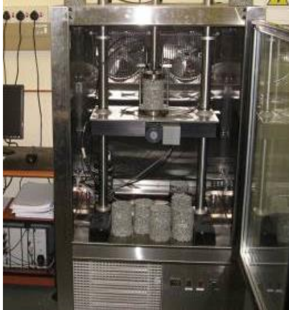
Figure 1: Test Specimens in a Temperature Chamber for Conditioning
