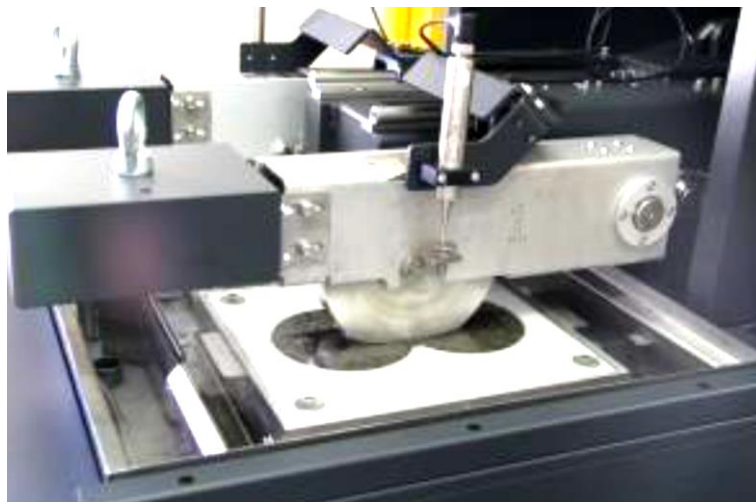
Figure 3: Hamburg Wheel Tracking Testing Set-Up
