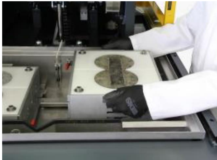
Figure 2: Specimens in Rutting Mould (After Testing)
