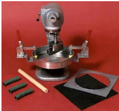
Figure E 41 Wet Track Abrasion Test Apparatus
