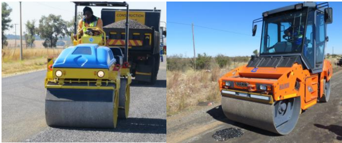
Figure F 5 Light and Heavy Steel Wheel Rollers
