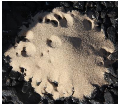
Figure E 12 Trickling of Sand into Surfacing Voids
