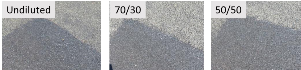
Figure H 20 Different Dilutions of Anionic Emulsions Applied
