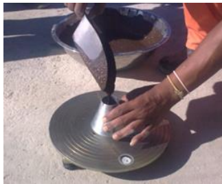
Figure E 52 ASTM Consistency Test
