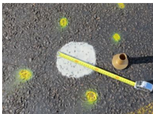
Figure A 3 Circular Sand Patch
