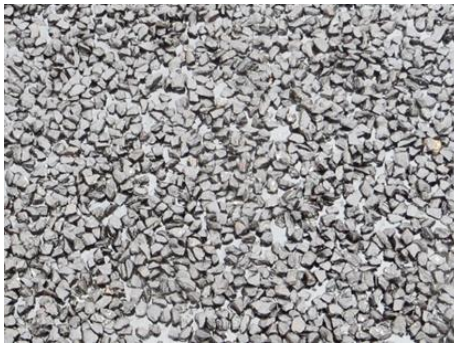
Figure F 31 Open Matrix after Rolling
