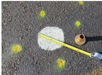
Figure E 10 Volumetric Texture Depth Measurement
