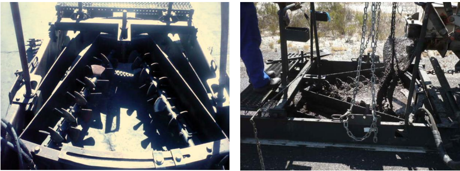
Figure F 10 Slurry Spreader Box for Rut Filling
