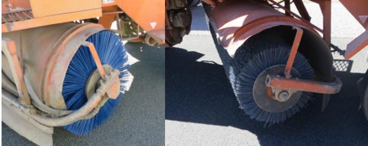
Figure F 7 New and Worn Bristles on a Rotary Broom
