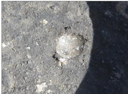
Figure E 5 Ball Penetration Test Indicating the “Half-Moon” Effect
