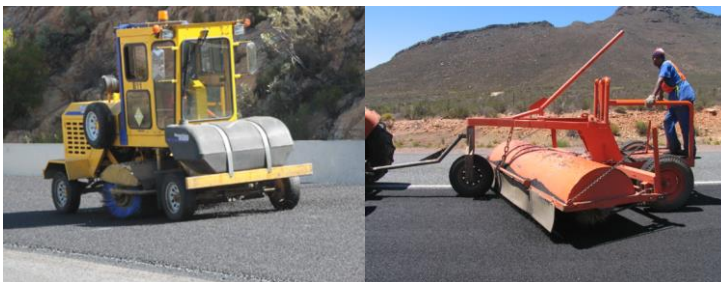
Figure F 6 Self-Propelled and Towed Type Rotary Brooms
