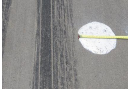
Figure D 20 20mm Cape Seal – Texture Depth 1.32
