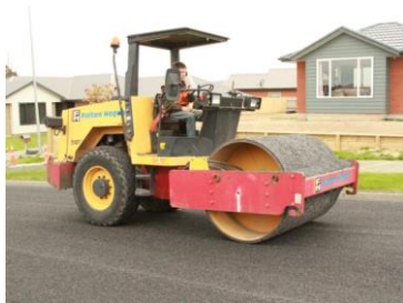
Figure F 4 Rubber Padded Steel Wheel Roller
