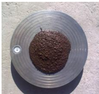
Figure E 53 Slurry Flow Measurement
