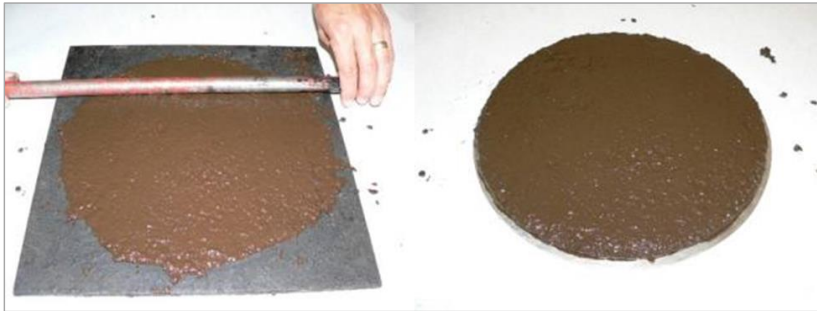
Figure E 43 Spread the Slurry Mix Evenly and Allow to Dry
