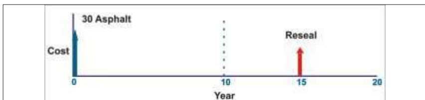
Figure 5 : Typical life-cycle strategy - 30 mm asphalt surfacing
