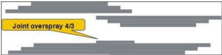
Figure 15: Centre line joint overspray
