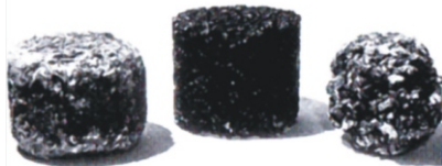
Results of Cantabro test: good performance (left) sample prior to testing (centre) and poor performance.
