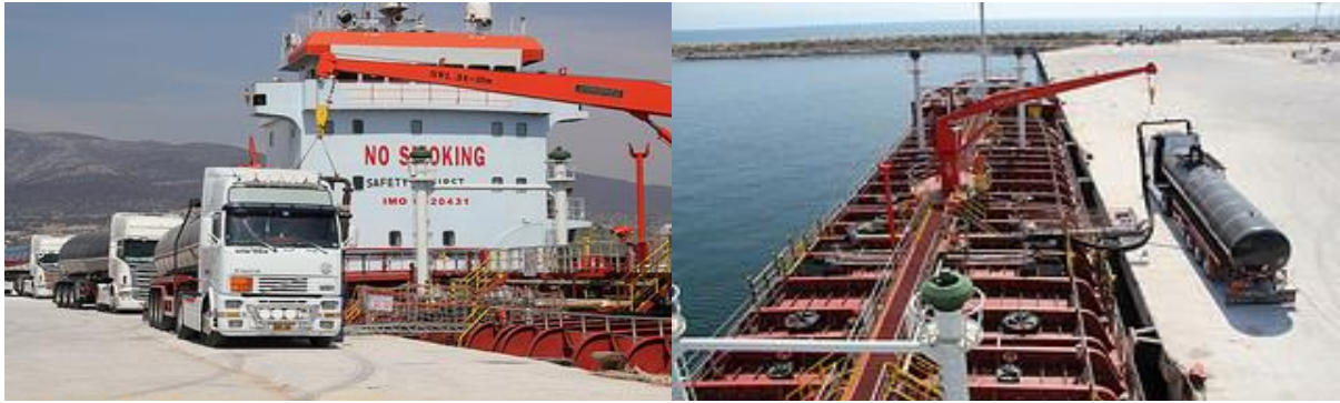
Figure 1A – Ship to shore arrangement to discharge bitumen directly to road tankers
