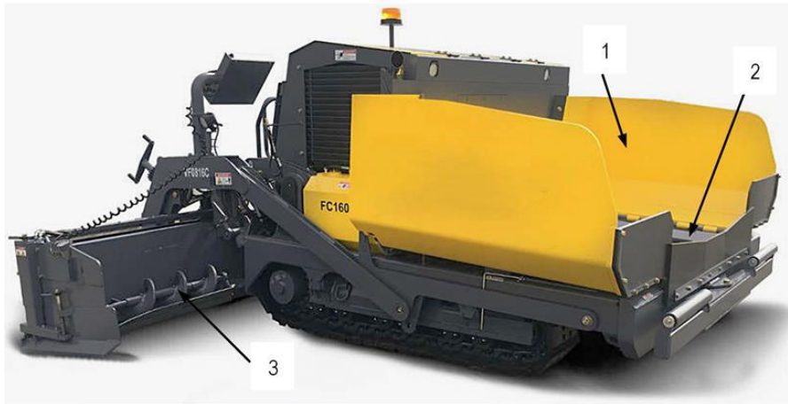
Figure 23: Asphalt Paver Feed System
