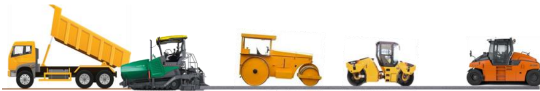
Figure 35: Paver and Compaction Train
