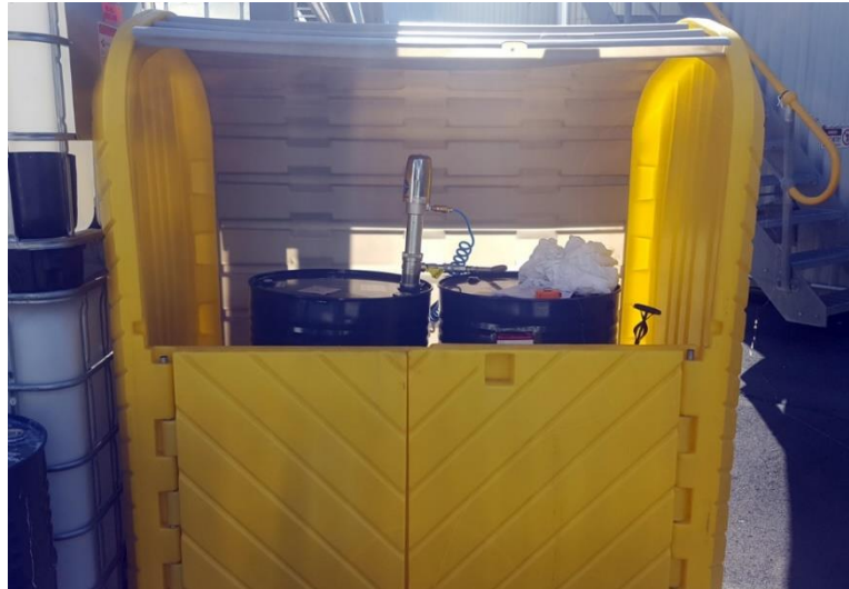
Figure 1. A permanent scavenger addition system with two drums of scavenger attached to a drum pump within stationary containment. (Image supplied and published with the kind permission of Road Science, Bay of Plenty, New Zealand)
