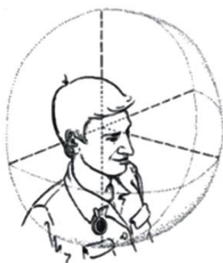
The breathing zone - a hemisphere of 300mm radius extending in front of a person's face measured from the mid-point of an imaginary straight line joining the ears.
