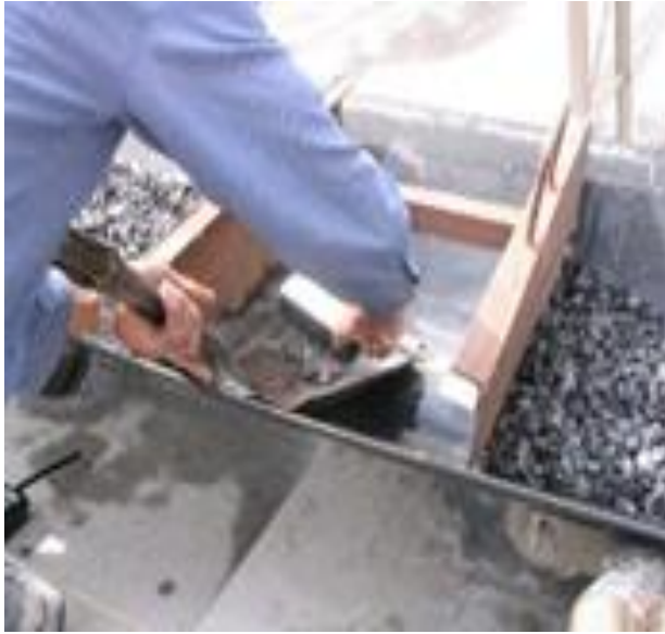
Brushing all fines remaining on conveyor belt
