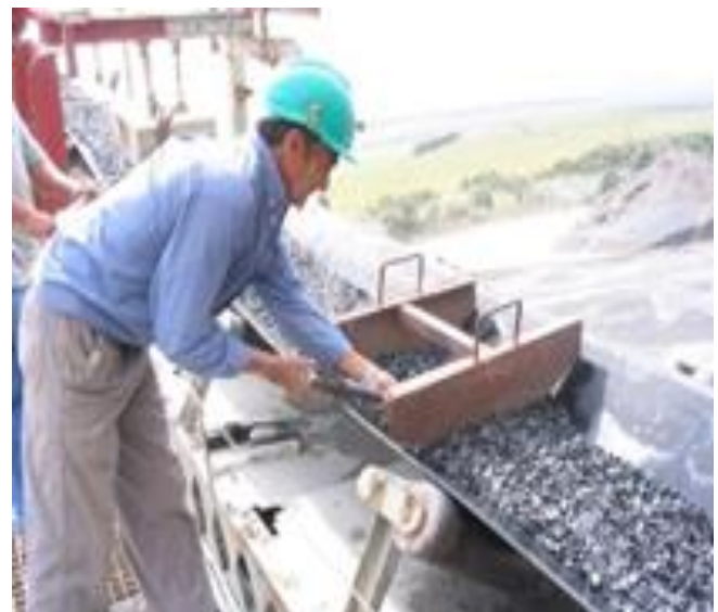
Commencement of sample extraction from conveyor belt
