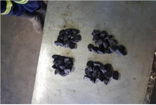
Photo 7 - Dividing material into four quadrants
