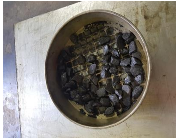
Photo 4 - Extra-large size particles on sieve being prepared for sub-division by coning and quartering
