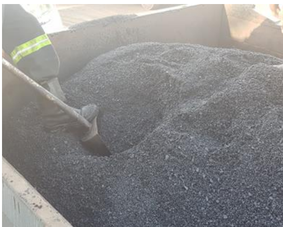
Figure A6: Using a Scoop-Type Shovel, the Sample is Procured
