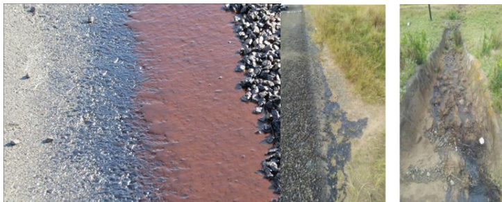
Figure C 30 Run-Off of Low Viscosity Emulsions
