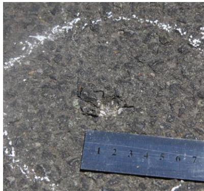
Figure E 8 Ball Penetration Test Indicating the “Crushing and Displacement” Effect
