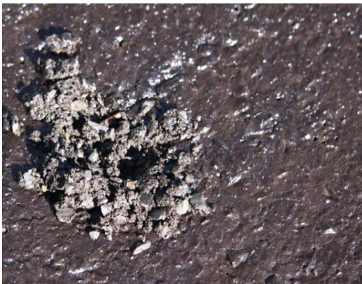
Figure F 38 Emulsion Segregated from Slurry Mix due to Too Early Rolling
