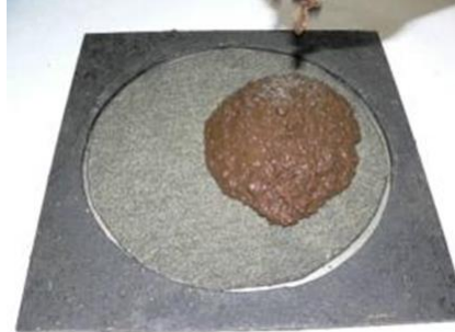
Figure E 42 Slurry Poured onto 300mm Felt Material
