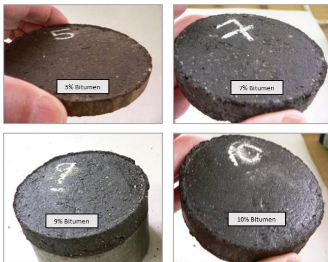
Figure E 48 Briquettes with Different Binder Contents (% Bitumen)
