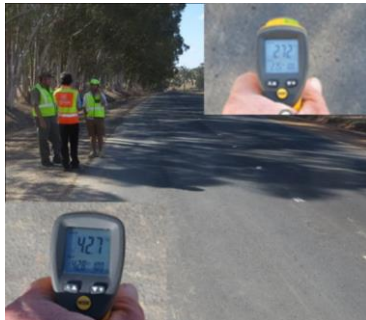
Figure E 21 Temperature Differences (Shade Versus Sun)
