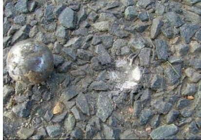
Figure E 6 Ball Penetration Test Indicating the “Crushing” Effect
