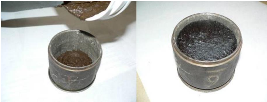
Figure E 38 A 20mm Layer of Slurry Poured into the Mould
