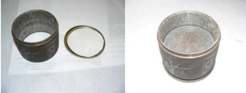
Figure E 37 Marshall Mould and Spacer for Mechanical Compaction
