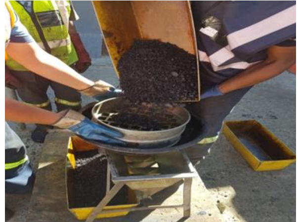
Photo 2 - Sieving extra-large particles
