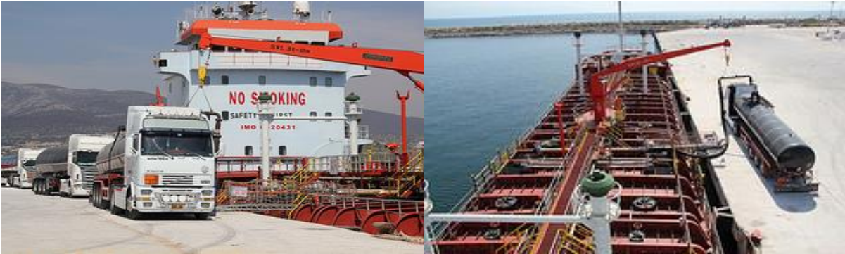
Figure 1 – Ship to shore arrangement to discharge bitumen directly to road tankers (Images courtesy of Atlantis Bitumen and Energy S.A.)
